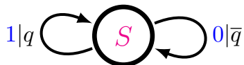
FIG. 5. Hägg-machine for the IID Process. When q = 1 , the IID Process generates a string of 1s, which is physically the 3C^+ stacking structure. Conversely, when q = 0 , the structure corresponds to the 3C^- structure. For q = 1/2 , the MLs are stacked as randomly as possible.
