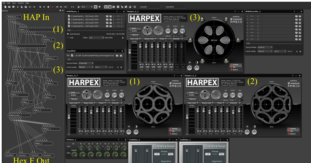
FIG. 3: Spatial Audio Processing Chain: Multi-HarpeX configuration within AudioMulch VST host for processing HAP first-order (4 channel) ambisonic A-Format hydrophone signals (HAP In) to Hexagonal F 6.1 surround format (3), using beamforming (1) and (2) to increase the directionality of the decoded Ambisonic signals and to steer away extraneous sound sources.
