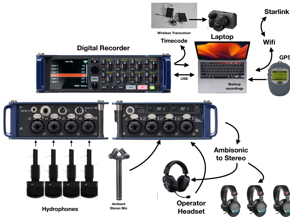
FIG. 4: First-order Ambisonic Recording and Observation System.
