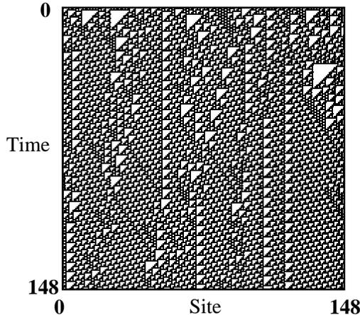
Figure 2: A space-time diagram illustrating the typical behavior of elementary CA (ECA) 110. The lattice of 149 sites, displayed horizontally at the top, starts with  $\mathbf{s}_0$  being an arbitrary initial configuration. Cells in state 1 are displayed as black and cells in state 0 are displayed as white. Time increases down the page.
