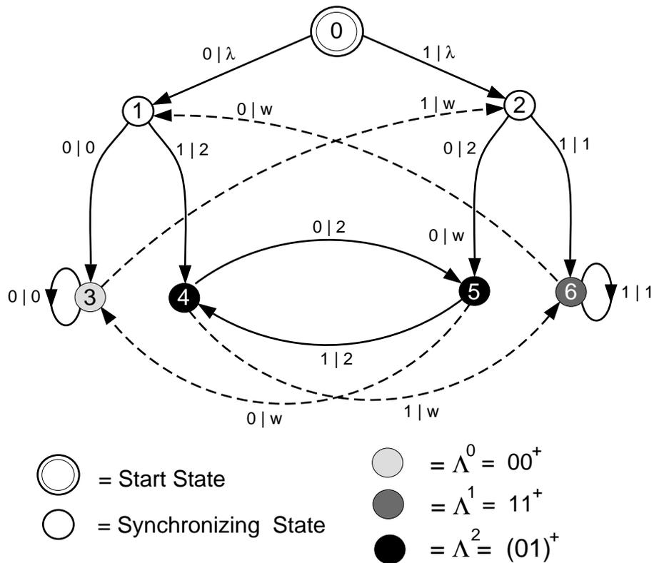
Figure 20:  $\phi_{\text{par}}^a$ 's domain-recognizing and filtering transducer. The edge labels  $s|t$  indicate that the transition is to be taken on reading configuration site value  $s \in \{0, 1\}$  and then outputting structural label  $t \in \{\lambda, 0, 1, 2, w\}$ .
