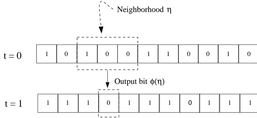
Figure 1: The components of one-dimensional, binary-state,  $r = 1$  (“elementary”) CA 110 shown iterated one time step on a configuration with  $N = 11$  lattice sites and periodic boundary conditions (i.e.,  $s_N = s_0$ ).
