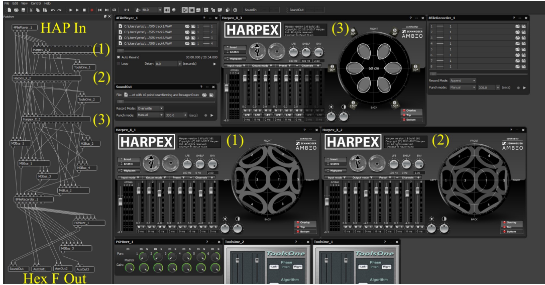
FIG. D.2: Spatial Audio Processing Chain: Multi-Harpex configuration within AudioMulch VST host for processing HAP first-order (4 channel) Ambisonics A-Format hydrophone signals (HAP In) to Hexagonal F 6.1 surround format (3), using beamforming (1) and (2) to increase the directionality of the decoded ambisonic signals and to steer away extraneous sound sources.
