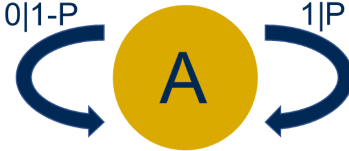
Fig. 6: Scheme of Biased Coin Machine(P: probability of defect at each site)
