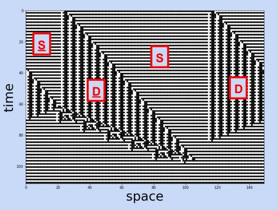
SS : create D domain SS : create D domain SD or SD : period 2, velocity 0 DS or DS : period 6, velocity 5/6 DS or DS : period 2, velocity -5/2 SD or SD : period 6, velocity 5/2 D / D interactions depend on relative phase
