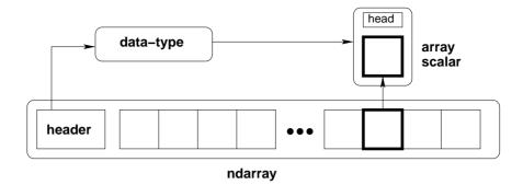
Figure 2.1: Conceptual diagram showing the relationship between the three fundamental objects used to describe the data in an array: 1) the ndarray itself, 2) the data-type object that describes the layout of a single fixed-size element of the array, 3) the array-scalar Python object that is returned when a single element of the array is accessed.
