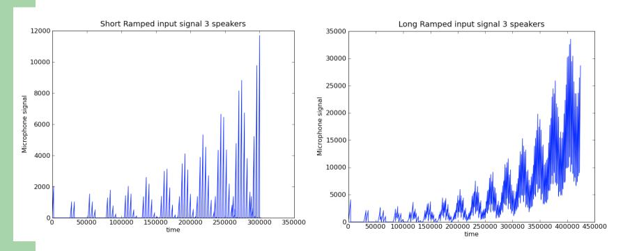
Duration of the ramped initial signal was doubled. Also note that the second chart was run longer.
